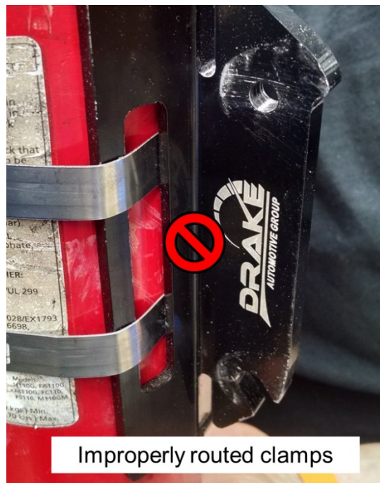
Figure B-48: Incorrect routing of hose clamps.
