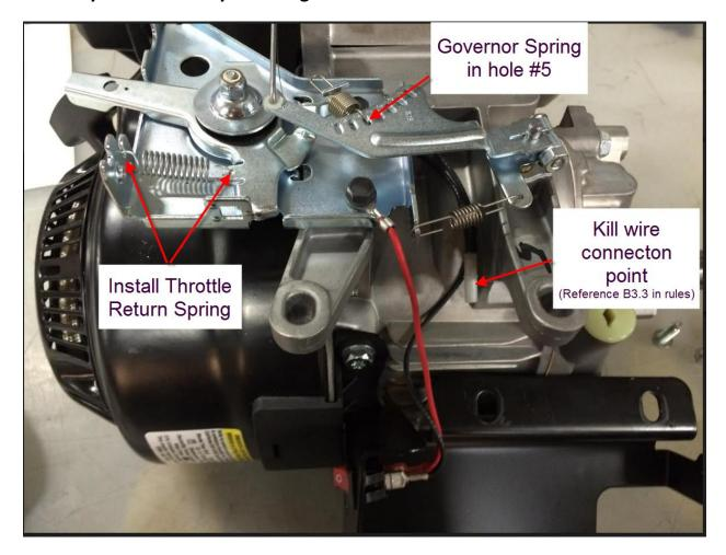
Install Throttle return spring in position shown above.
