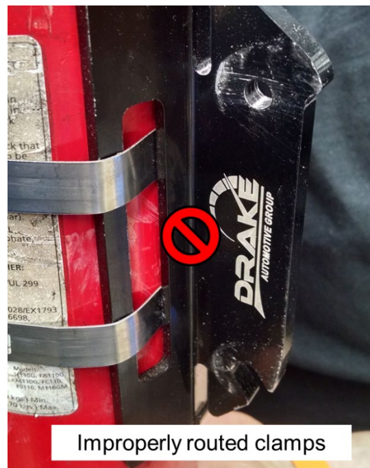
Figure B-52: Incorrect routing of hose clamps.
