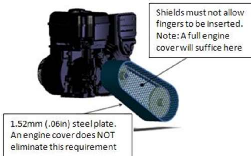
Figure B-48: Powertrain Guard Example
