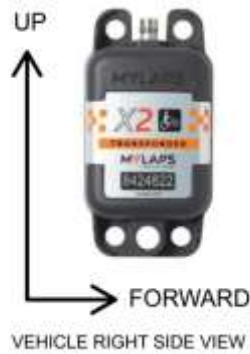
Figure B-57: Transponder Orientation
