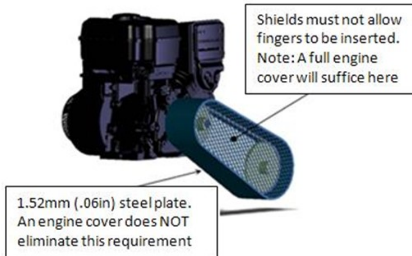
Figure B-51: Powertrain Guard Example
